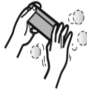
Clean the filter: blow out the dust. Change when too dusty or at 3 years old
